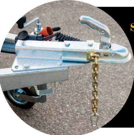
**Safety chains are a simple yet often overlooked towing aid. Every trailer should come with two safety chains which are intended to be crossed when attached to your vehicle.**
